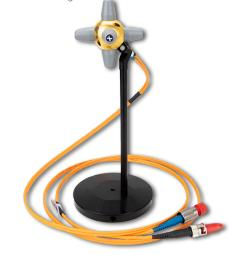
**Internal calibration data** The linearity adjustment data is by default stored inside the probe. In addition, the frequency response calibration data of the X-Y-Z axis can be stored as user correction data inside the probe. As a result there is no need to apply frequency dependent corrections for individual axis' in software anymore. This feature results in a high accuracy and ease-of-use.
